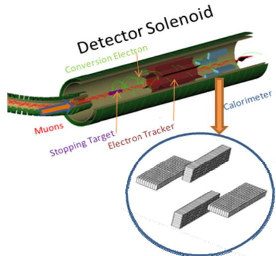
Figure 6: Mu2e detector. Electromagnetic calorimeter is shown in more detail. MPPCs could be used as photon detectors for the calorimeter.
