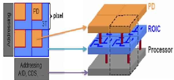
Figure 8: Correspondence of the functions of an optical detector using conventional 2D technology and one using 3D IC technology. The photon detector (PD), readout (RO) and processor functions are shown
