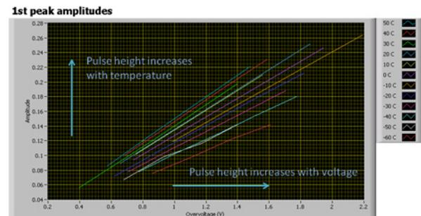
Figure 2: MPPC signal amplitude vs. overvoltage for temperatures between -60C and +60C. Overvoltage is the increase in bias voltage above the breakdown potential.
