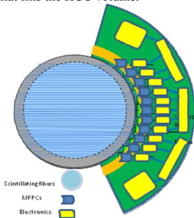
Figure 5: Layout of scintillators, MPPCs, and electronics for a typical detector plane in the MANX cooling channel.
