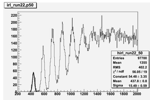
Figure 1: Output pulse height distribution from an MPPC interfaced to a plastic scintillator with a radioactive source. Note the clearly defined peaks corresponding to discrete numbers of photoelectrons.
