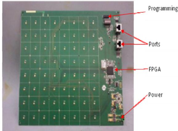
Figure 7: Array of 64 MPPCs mounted on the same board as the readout electronics.
