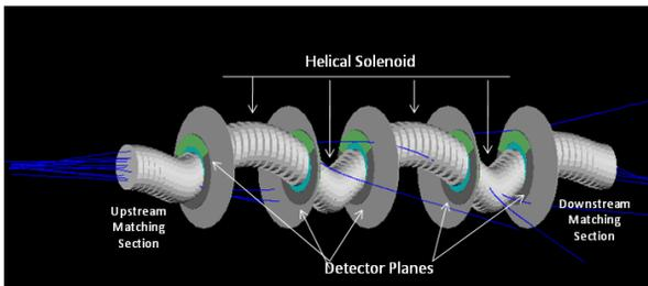
Figure 3: Schematic representation of the MANX cooling channel with 5 sets of trackers inside. The first tracker is mounted between the upstream matching magnet and the HCC, three trackers are built into the HCC coil structure, and the last tracker is between the HCC and the downstream matching magnet. The trackers alternate between x-y and u-v units.
