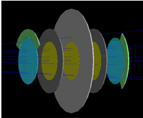
Figure 4: Exploded view of an x-y tracker unit. The central disk is a mounting plate that is permanently installed in the coil structure. Next are the detector support rings, and outer scintillators and electronics, which are built as units that are installed on the central mounting plate. The yellow disks represent liquid helium that fills the HCC volume.
