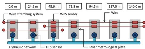
Figure 7: Layout of the TT1 facility.
