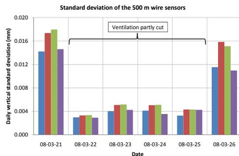
Figure 4: Standard deviations of the 500 m wire sensors.
