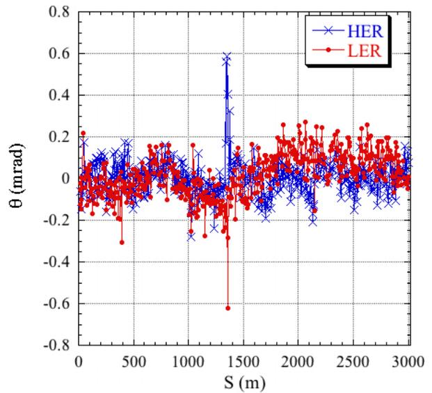
Figure 4: Quadrupole magnet tilt  $\theta$ . The average of two reference bases is plotted for each HER/LER magnet against  $s$ .
