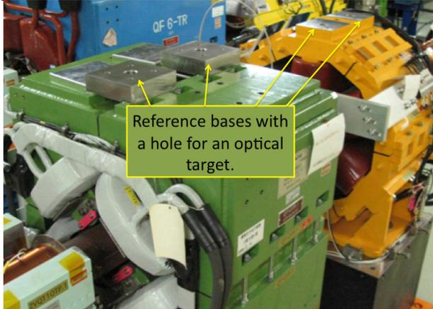
Figure 3: Magnet reference bases for alignment. There are two reference bases per magnet for defining the magnet axis along the beam line.
