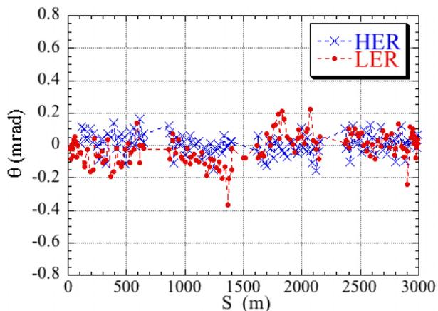
Figure 7: Dipole magnet tilt  $\theta$  vs.  $s$ .
