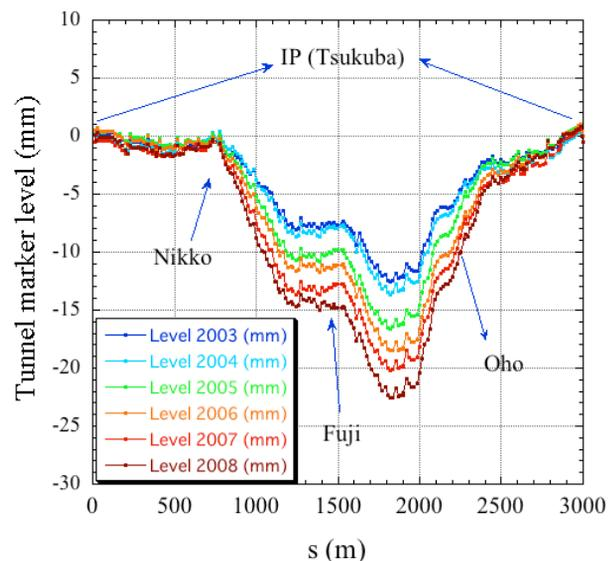
Figure 2: Marker positions measured along the tunnel.
