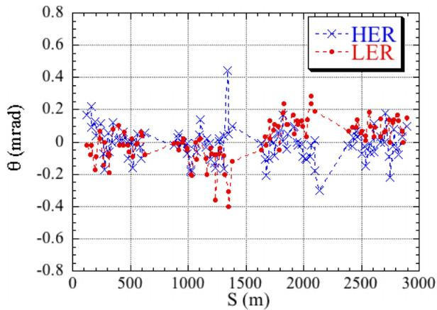
Figure 6: Sextupole magnet tilt  $\theta$  vs.  $s$ .
