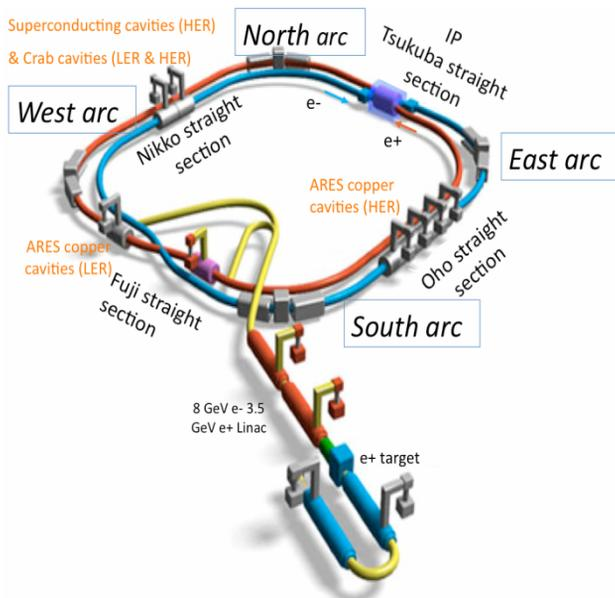
Figure 1: KEBB tunnel. The 8 GeV electron beam circulates clock-wise and the 3.5 GeV positron couterclock-wise.
