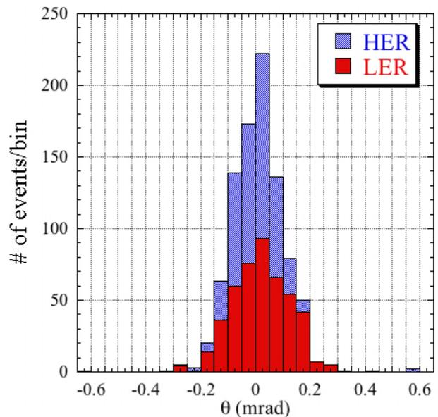
Figure 5: Histogram of magnet tilt  $\theta$  for HER and LER quadrupole magnets.
