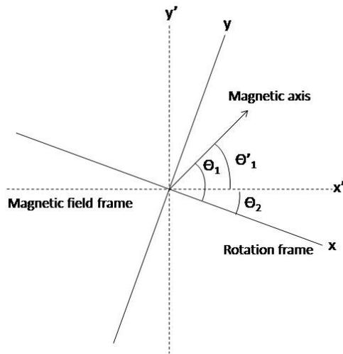
Figure 2: Rotation and magnetic field coordinate systems.
