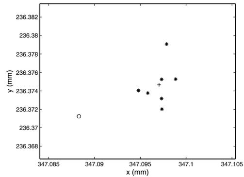
Figure 5: Magnetic center of the quadrupole magnet (\*). The plus sign is the mean value of the seven measurements and the circle corresponds to the geometrical center.
