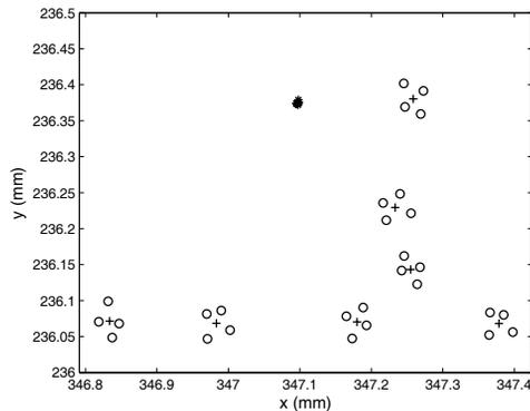
Figure 4: Magnetic center measurements. Circles are the geometrical axis of the steel shaft, + is the axis of rotation and \* is the magnetic center. The area around the magnetic center is enlarged in figure 5.
