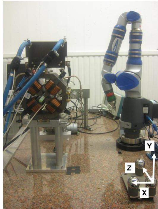
Figure 3: Platinum Faro arm and metal spheres defining the coordinate system.
