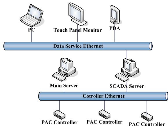
Figure 3: Network structure of the vibration measurement system.
