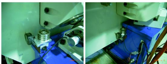
Figure 6: Position of a dial gauge.
