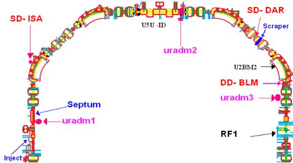
Figure 1: One half of the VUV ring, after the injection septum showing the magnets and BLM's.
