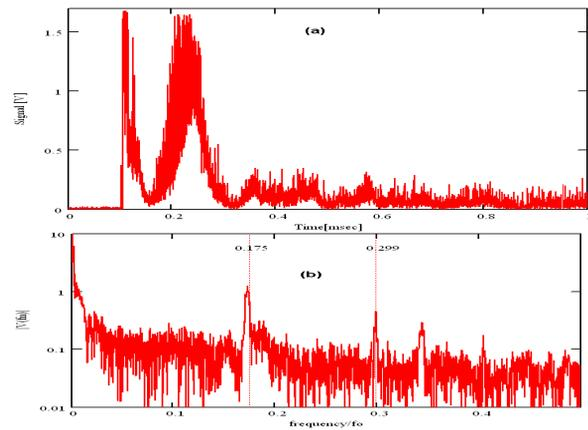
Figure 4: (a) SD-ISA injection loss signal vs time (1msec FS) in 2006 and (b) FFT of the signal in (a) scaled by  $f_0$ .
