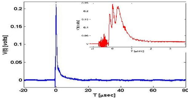
Figure 5: Present SD-ISA injection loss signal vs. time after momentum offset correction. Inset shows details of the pulse (stored and injected beam) during the 3 turn bump.
