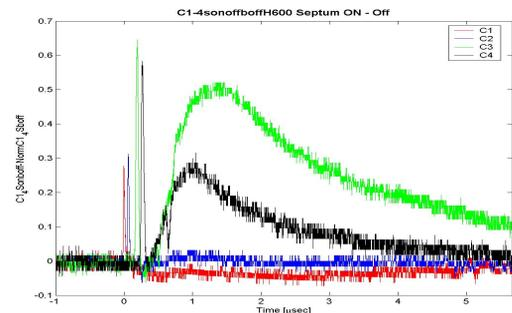
Figure 7: SD signals in the Xray injection period (C1, C2) compared to next period (C3, C4) for the septum on minus the septum off condition.
