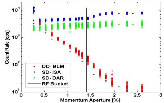
Figure 6: DD, ISA and DAR PCR's shown as the horizontal scraper reduces the ring momentum aperture.
