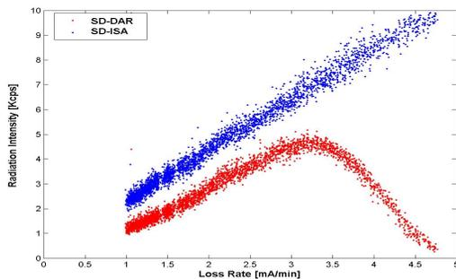
Figure 2: The PCR versus beam loss rate ( $I_0/\tau$ ) of the VUV ring for the two SD's during several operational fills.
