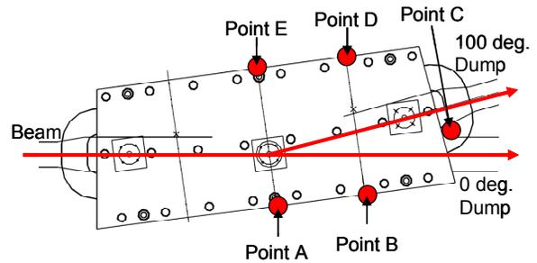
Figure 7: Points for Residual Radiation on Bend Magnet.
