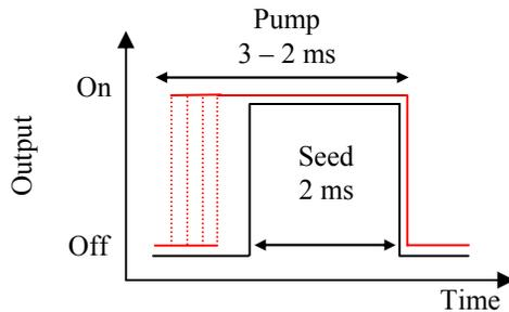
Figure 3: Burst temporal structure.
