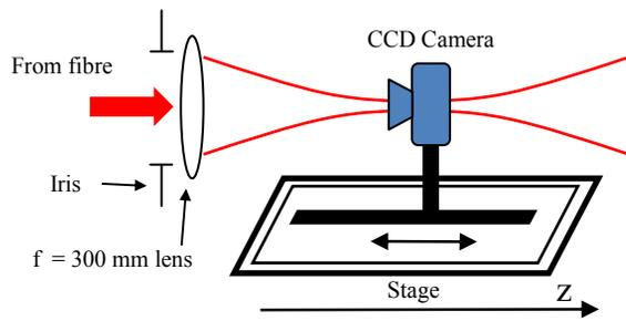
Figure 2:  $M^2$  measurement system.
