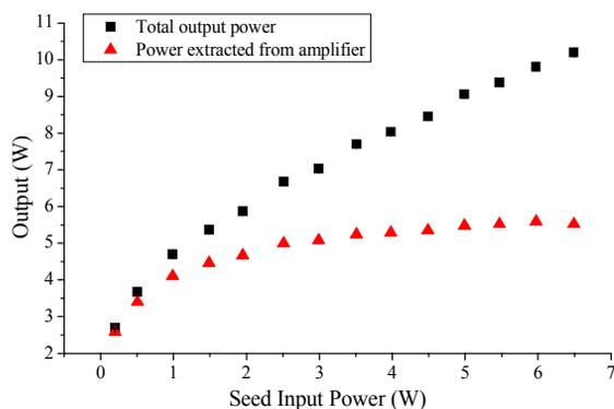
Figure 7: Output power with a variable input power.
