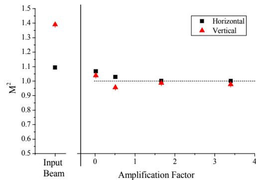
Figure 4:  $M^2$  at various levels of amplification.
