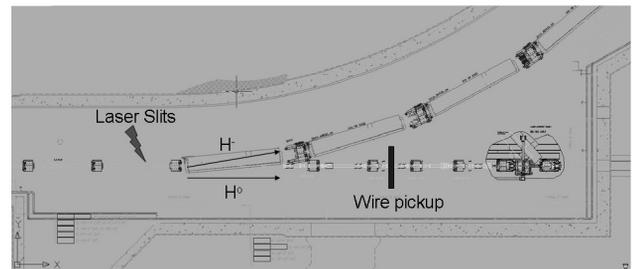
Figure 2: Schematic plot of the 1 GeV laser emittance scanner to be installed in HEBT of the SNS. Stripped  $H^0$  beam goes straight while  $H^-$  beam travels along the bending dipole separating two species.
