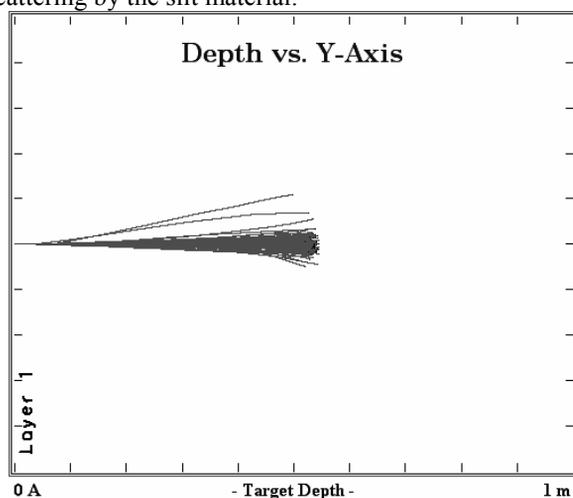
Figure 1: Plot of the stopping range of a 1-GeV beam in solid copper. The range of the horizontal axis is 1 m.
