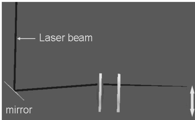
Figure 3: Schematic plot of the laser slit of the emittance scanner.
