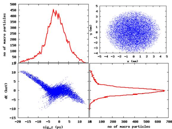
Figure 6: Longitudinal phase space and transverse beam cross-section of the bunch at the first cell of SC structure.
