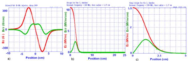
Figure 4: a) Max. magnetic field of solenoid, b) Normalised Electric field components of SHB, c) Normalised Electric field components of FB.
