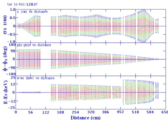
Figure 5: Beam envelope, bunch length and energy spread variations along the injector for 120 pC bunch charge. SC module starts at 577 cm.
