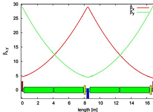
Figure 3: Beta functions in a cell of the FODO lattice and sketch of a single FODO cell.
