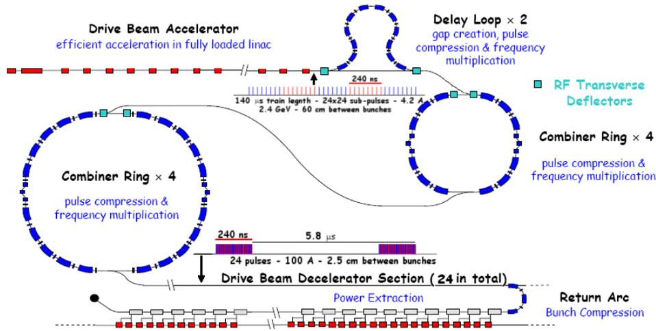
Figure 1: Schematic layout of one CLIC RF power source complex.
