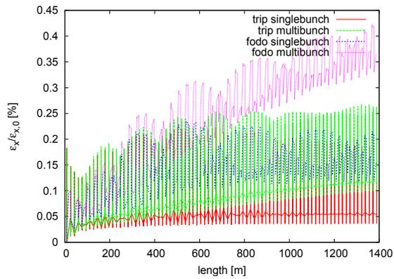
Figure 4: Emittance variation along the linac for triplet and FODO lattice.
