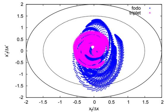
Figure 6: The amplification factor of the beam at the end of the drive-beam accelerator, using the FODO and triplet lattice.  $\Delta x$  and  $\Delta x'$  is initial beam offset of the beam;  $x_f$  and  $x'_f$  final beam coordinates.
