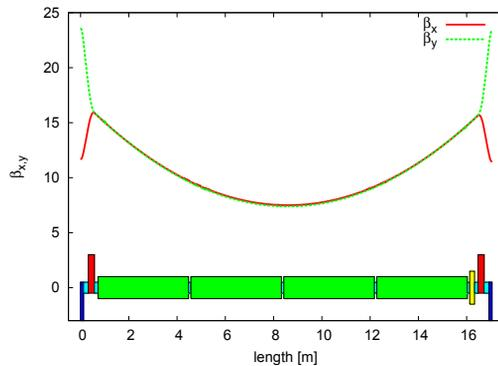
Figure 2: Beta functions in a cell of the triplet lattice and sketch of a single triplet cell.
