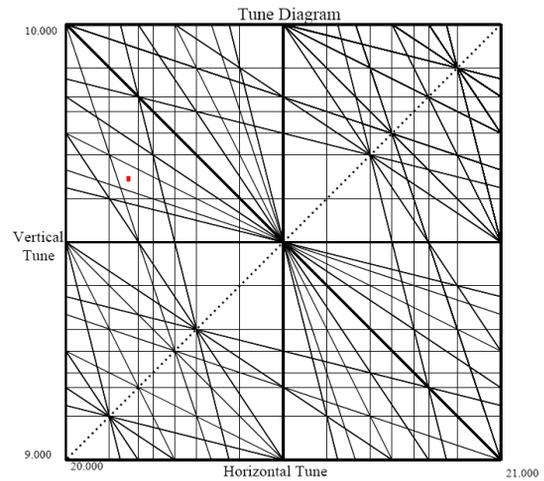
Figure 4. Tune diagram of DDBA lattice.
