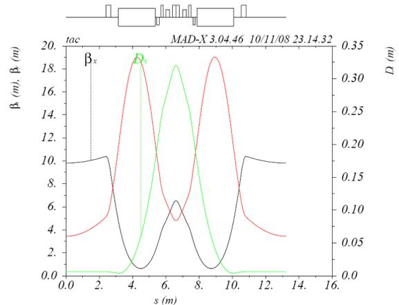
Figure 1: Lattice functions for 23 periods DBA lattice
