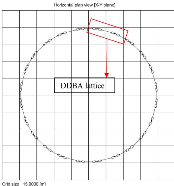
Figure 6: The schematic of the full storage ring with DDBA lattice.
