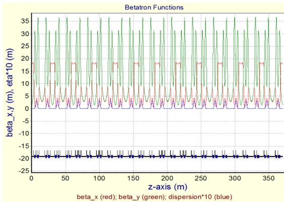
Figure 5: Lattice functions for the full storage ring with the DDBA.
