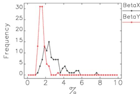
Figure 3: Histogram of the relative beta function error rms after beta function correction.
