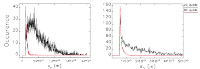
Figure 6: Left – histogram of effective vertical emittance at ID locations; right – histogram of vertical beam sizes at the same points. Black curve corresponds to correction with 20 skew quadrupoles, red curve – with 80 skew quads.
