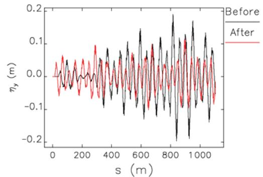
Figure 5: An example of vertical dispersion before and after correction.
