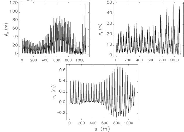
Figure 1: Typical beta functions before beta function correction. Top left – horizontal, top right – vertical, bottom – dispersion.
