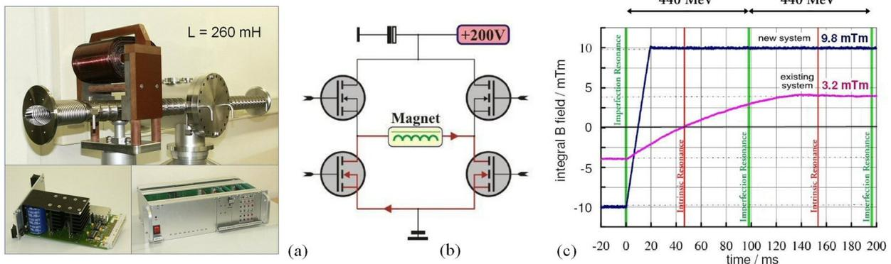
Figure 5: (a) New steerer magnet and beam pipe (top), H-bridge and complete power supply (bottom). (b) Schematic of the pulsed H-bridge, indicating the inductance-driven current loop between two consecutive loading pulses (lower section). (c) Comparison between existing setup and new system (at 4.5 GeV/sec ramping speed).
