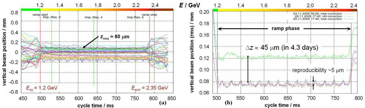
Figure 3: Closed orbit correction during the fast energy ramp: (a) Development of the vertical beam position at each BPM (bold line: rms). (b) Long term stability and reproducibility of the vertical closed orbit rms.
