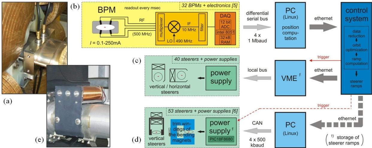
Figure 2: (a) BPM fixed to the center of its quadrupole magnet. Schematic overview of the BMP and the readout (b) as well as the correction scheme for the existing setup (c) and the new system (d). Existing steerer magnet (e).
