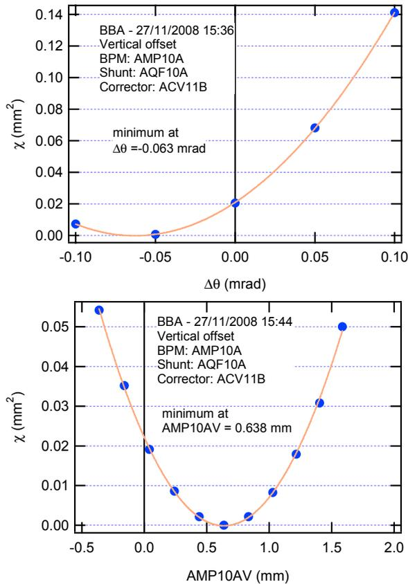
Figure 1: Coarse (top) and fine (bottom) iterations for BBA measurements to determine the vertical offset of BPM AMP10A.
