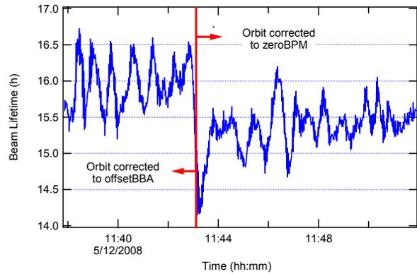
Figure 4: Decrease in beam lifetime by switching the reference orbit from offsetBBA to zeroBPM.
