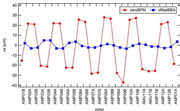
Figure 3: Horizontal orbit distortion induced by a variation in chromaticity for offsetBBA and zeroBPM orbit references.
