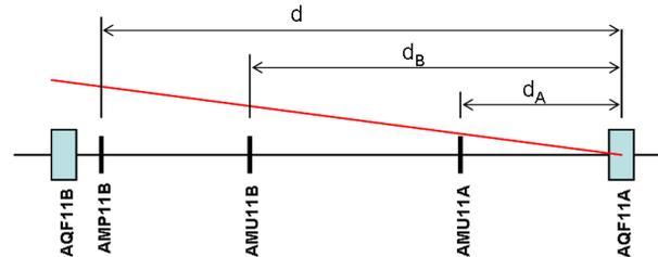
Figure 2: Schematic diagram of BPMs in the undulator section.
