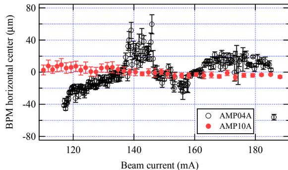
Figure 5: BBA measurements to compare the horizontal drift with current of a new type of button BPM (AMP10AH) with the old stripline type (AMP04AH).
