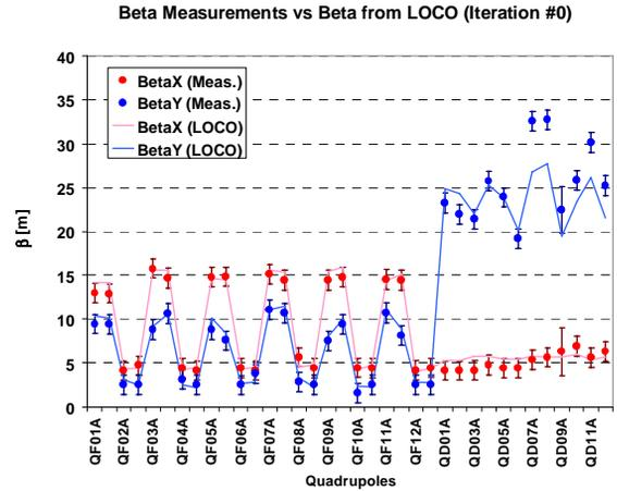
Figure 3: Comparison between measured beta functions and beta functions from LOCO-calibrated ring model.
