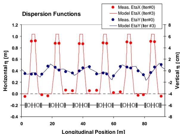
Figure 5: Comparison of measured dispersion functions (symbols) before symmetrization with corresponding functions given by the model after symmetrization (lines).
