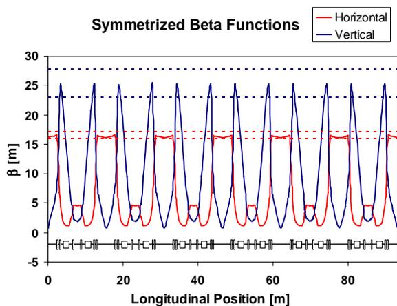
Figure 4: Beta functions for the symmetrized optics as determined from orbit response matrix measurements. Dashed lines show intervals within which lied maxima of the original beta functions.
