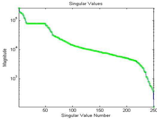
Figure 2: LOCO singular value spectrum for the coupled response matrix fit.
