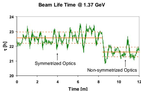
Figure 6: Improvement of beam lifetime with symmetrization.
