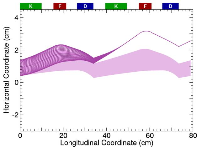
Figure 4: Injection of a 20 MeV beam into EMMA. Everything is as in Fig. 3, except only the 20 MeV circulating beam is shown.
