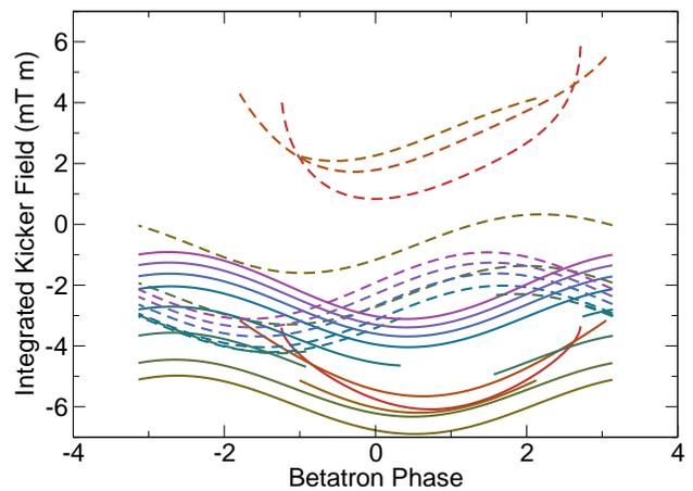
Figure 8: Integrated kicker fields for different betatron phases on the 3 mm normalized horizontal ellipse. Different colors are for different energies. Solid lines are for the kicker closest to the septum, dashed are for the other.
