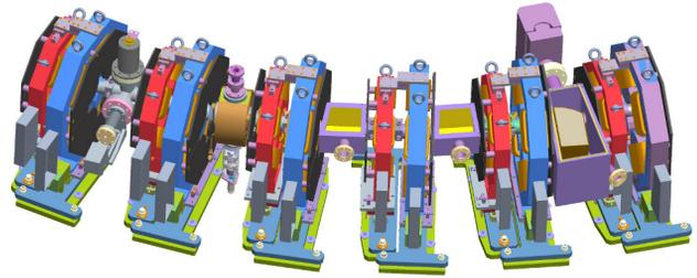
Figure 1: Injection region of EMMA, showing, right to left, the injection septum and two kickers.
