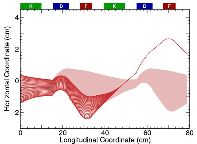
Figure 6: Extraction of 10 MeV beam from EMMA. The beam goes from left to right in the drawing. The last point plotted on the right is where the beam enters the septum. Only the 10 MeV circulating beam is shown. Everything else is as in Fig. 3.
