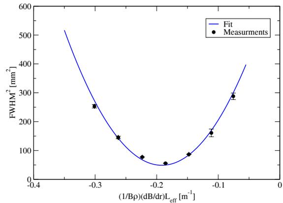
Figure 5: Emittance scan using BtA Q1.
