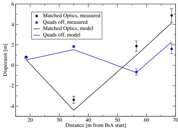
Figure 4: Dispersion measurements and model predictions.
