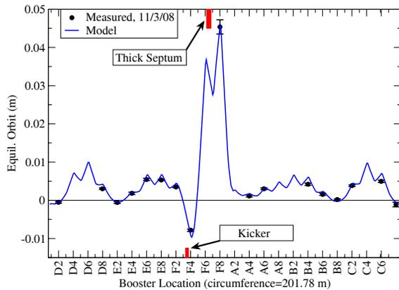
Figure 1: Booster extraction orbit distortion.
