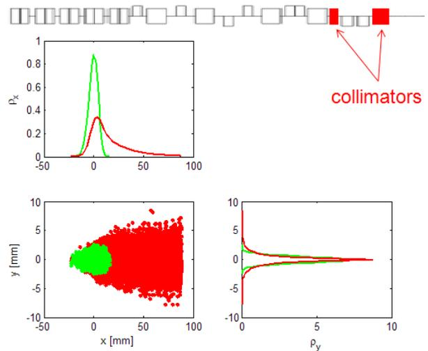
Figure 5: Location of collimators (upper plot) and high (red) and low (green) energy spread beams on the dump window (lower plot).
