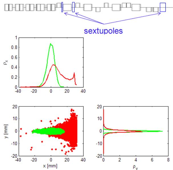
Figure 2: Location of strong sextupoles (upper plot) and 3.54% (red) and 0.15% (green) energy spread beams on the dump window (lower plot).
