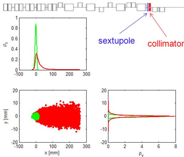
Figure 4: Location of sextupole and collimator (upper plot) and high (red) and low (green) energy spread beams on the dump window (lower plot).
