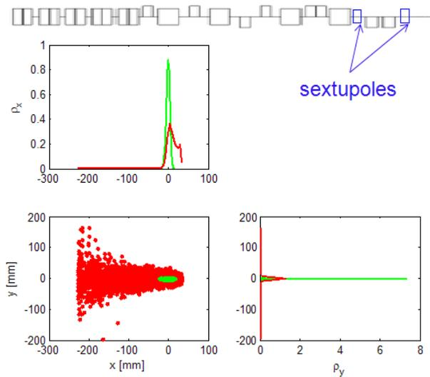
Figure 3: Location of sextupoles (upper plot) and high (red) and low (green) energy spread beams on the dump window (lower plot).
