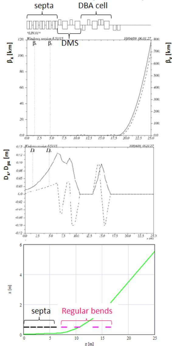
Figure 1: Twiss parameters and dispersion (two upper plots), and beam trajectory (lower plot) in ELBC.
