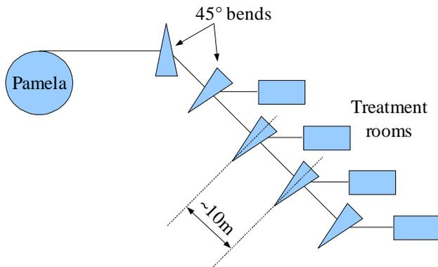
Figure 1: Proposed layout of the transport line.
