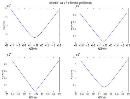
Figure 3: Horizontal & vertical IP beam sizes  $\sigma_x$  &  $\sigma_y$  vs QD0 & QF1 strengths for the 20,100 times  $\beta_{x,y}$  ATF2 optics.
