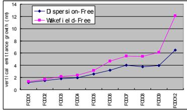
Figure 11: vertical emittance growth after wakefield-free steering and dispersion-free steering.
