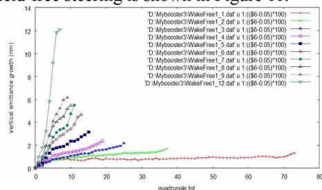
Figure 10: vertical emittance growth after wakefield-free steering including cavity, quadrupole and BPM misalignment (include initial energy spread).
