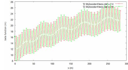
Figure 7:  $\beta$  functions of FODO1 versus the longitudinal position (green:  $\beta_y$ ; red:  $\beta_x$ ).
