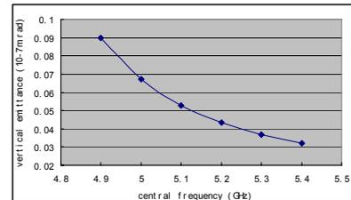
Figure 13: vertical multi-bunch emittance versus central frequency by gauss-frequency detuning ( $\delta y_0 = 10 \mu\text{m}, \text{nb} = 312$ ).
