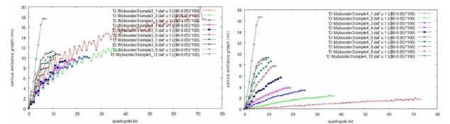
Figure 9: vertical emittance growth including cavity and BPM misalignment after one-to-one correction (left: initial energy spread included, right: without initial energy spread).
