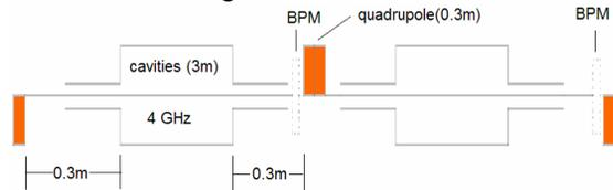
Figure 1: Layout of one FODO cell.
