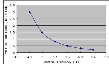
Figure 12: vertical multi-bunch emittance versus central frequency by two-frequency detuning ( $\delta y_0 = 10 \mu\text{m}, \text{nb} = 312$ ).
