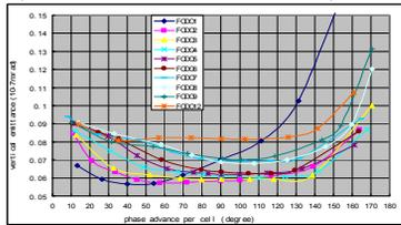
Figure 3: vertical emittance growth versus quadrupole strength and different number of accelerating structures per cell ( $\delta\text{yc}=100\mu\text{m}$ ).
