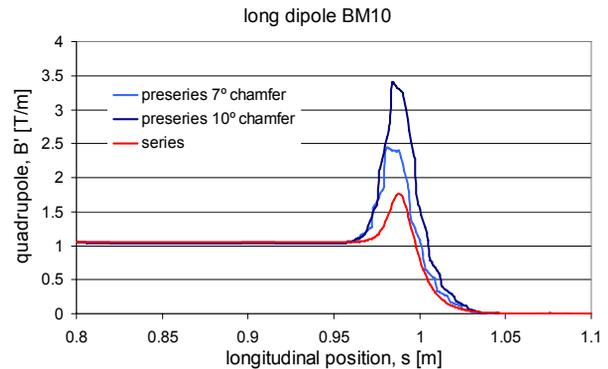
Figure 1: The quadrupole profile in the fringing region of the long dipole. The peak value measured on the series (red line) is about a factor two below the needed value (chamfer cut between 7° and 10°).
