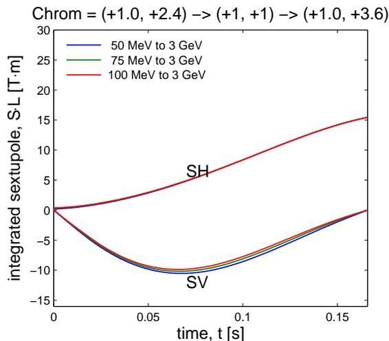
Figure 5: The SH and SV sextupole tracking with dipole ramping starting at different energies. The sextupole power supplies tracking to keep the chromaticities higher than +1 is performed in the minimum range in order to have the largest dynamic aperture all along the ramping.
