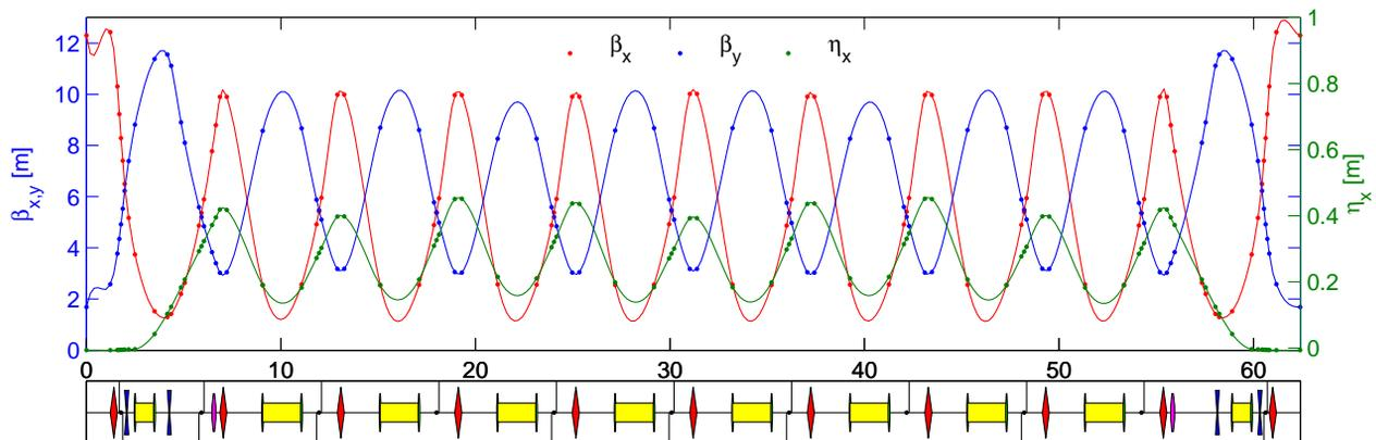
Figure 2: Beta and dispersion functions in one arc of the machine, matched according to the measured magnets. The quadrant composes of 8 unit cells with long dipole and focusing quadrupole, and 2 matching sections with short dipole and three quadrupole families. The sextupole families are located in the dispersive section next to the short dipoles.
