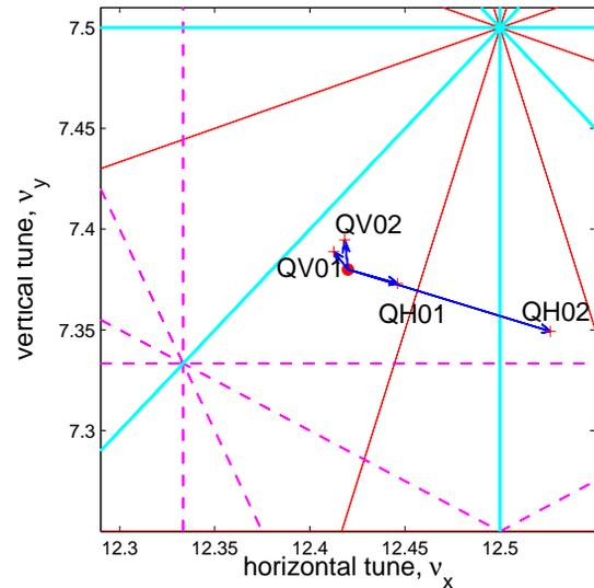
Figure 3: Nominal working point (12.42, 7.38) and tune shifts due to a strength change  $\Delta k = 0.01$  in the four quadrupole families. The resonance lines up to 4<sup>th</sup> order are plotted.
