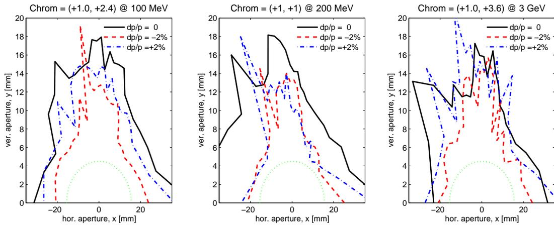
Figure 4: Dynamic apertures compared with the vacuum chamber physical acceptance at injection (leftmost), maximum eddy current effect (centre), and extraction (rightmost).
