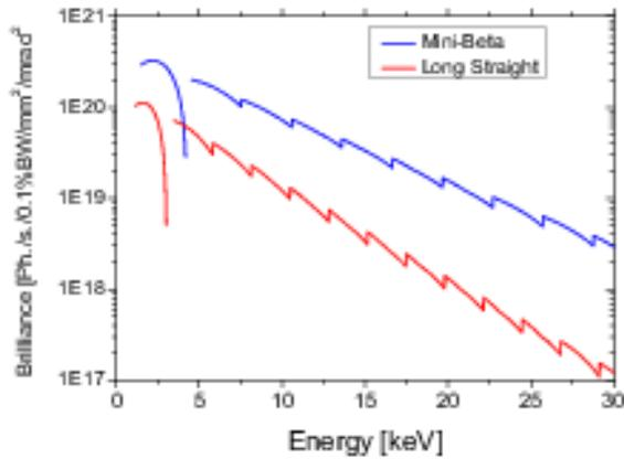
Figure 2: Comparison of a 3m long U20 cryo-cooled undulator (blue) in a mini-beta section and a comparable undulator in a long straight (U28).
