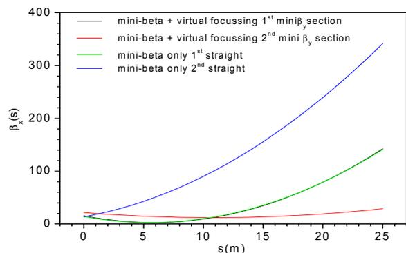
Figure 1: comparison of the virtual  $\beta_x$  downstream beamline between ‘two mini  $\beta_y$  + virtual focussing’ and ‘two mini  $\beta_y$ ’ optics
