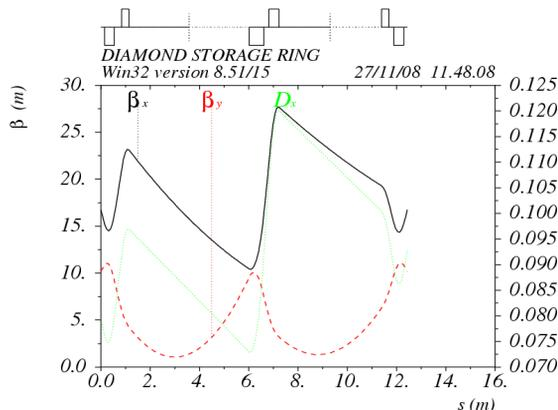
Figure 3: Optics functions in modified long insertion straight.
