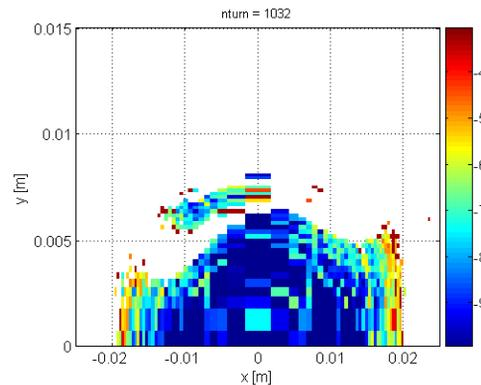
Figure 4a: DA computed with I13 modification with 1% coupling generated by roll off quadrupoles.
