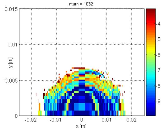
Figure 5: DA with I13 and I09 optic and 1% coupling.
