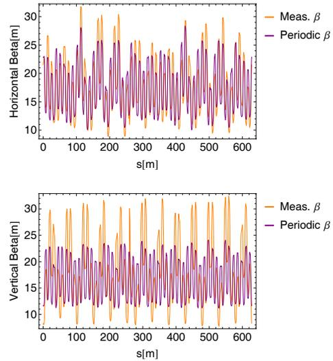
Figure 6: Horizontal and vertical measured beta-functions shown with the periodic beta at PS injection
