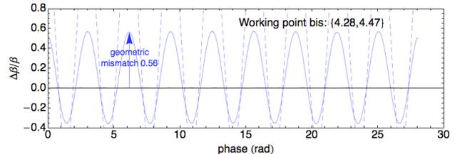
Figure 3: Beta-beating with the initial injection chicane (dashed) and after increasing the magnetic length and decreasing the deflection angles.
