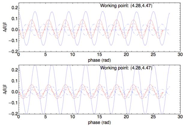
Figure 4: Beta-beating with passive compensation of perturbations due to the chicane by rotating BS pole faces by 44 mrad (upper image) and 33 mrad (lower image) for three different deflections 66 mrad (solid), 44 mrad (dashed) and 22 mrad (dot-dashed)
