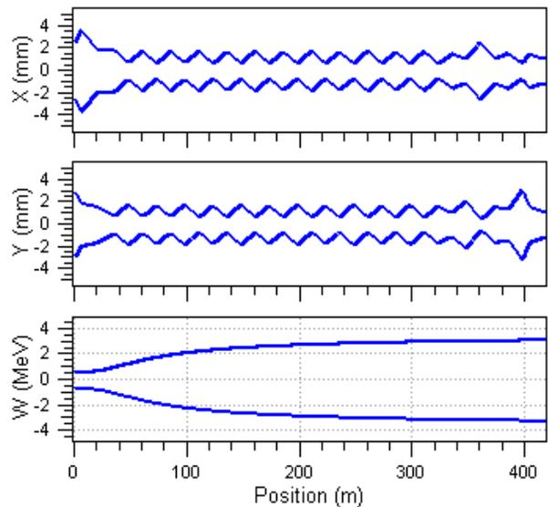
Figure 4: Envelopes in the horizontal (top) and vertical (middle) planes plus the beam energy spread (bottom) evolution along the beam line with a current of 62 mA.
