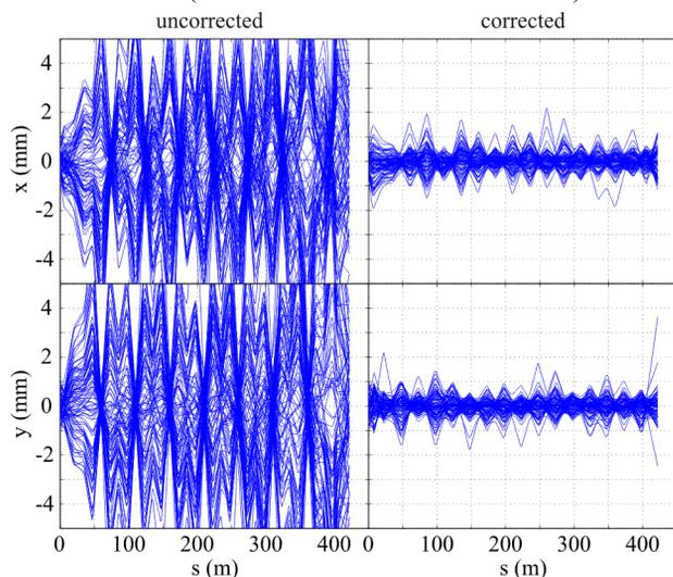
Figure 5: Plot of 100 uncorrected and corrected trajectories for the combined 1-in-1 / 2-in-3 scheme.
