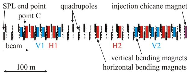
Figure 2: Beam line layout of the SPL-PS2 transfer line. A FODO lattice with 90° phase advance per cell and four families of bending magnets is being used.
