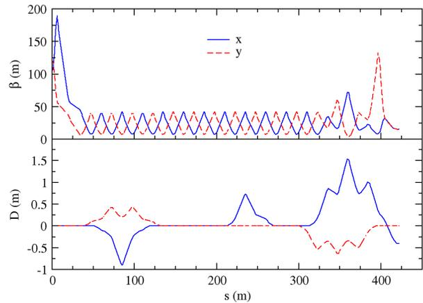
Figure 3: Simulated beta and dispersion functions along the SPL-PS2 transfer line for a 4 GeV H<sup>-</sup> beam using MAD-X.
