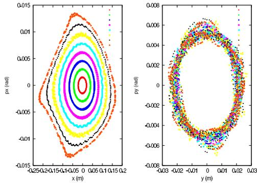
Figure 6: The meaning of the plots is the same as in Fig. 5 but the ring is now equipped with sextupoles to correct for chromaticity effects (see text). This results in highly non-elliptical trajectories (Poincaré plot on the left) and coupling between  $x$  and  $y$  planes, as can be inferred from the blurred trajectories.
