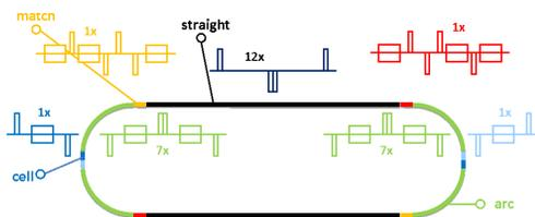
Figure 1: Schematic diagram of the Race Track Decay Ring with its main regions: (black) decay straights, (green/blue/cyan) arc sections, (red/yellow) matching sections. The small diagrams show the structure of the linear optics cells.
