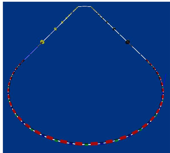
Figure 8: A perspective view of the Race Track Decay Ring in G4Beamline. Color convention: (red) dipoles, (blue) focussing quadrupoles, (green) defocussing quadrupoles, (yellow) virtual detectors for tracking studies.
