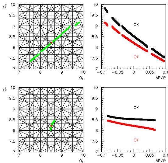
Figure 4: Upper section: linear optics configuration. (Left) tune excursion with crossing of resonances as a function of momentum displacement (green line): the red dot shows the working point. The natural chromaticity of the beam is shown on the right for both the transverse planes. Lower section: the effect of sextupoles is shown. Chromaticity is strongly reduced (right) and also the crossing of potentially dangerous resonances.
