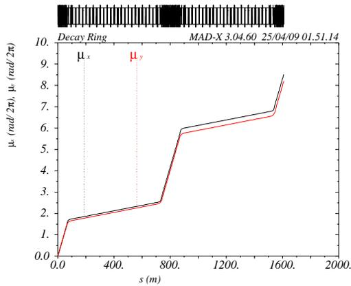
Figure 3: Phase advance over a period in the Decay Ring with a fast increase in the arcs due the small beta functions and a slow increase in the straights where  $\beta_{x,y}$  are large.
