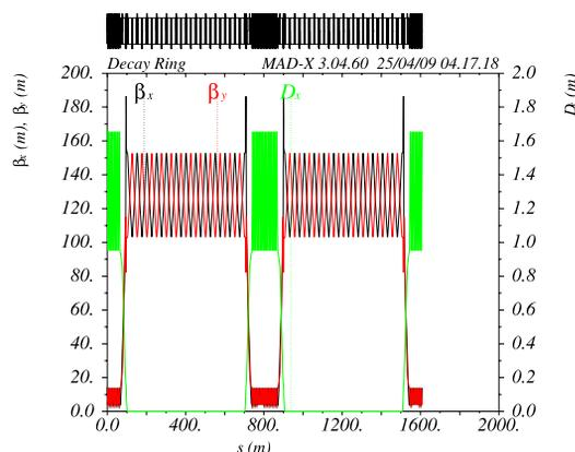
Figure 2:  $\beta_x$  (black) and  $\beta_y$  (red) functions for the decay rings. Their values are deliberately chosen high in the straight sections to reduce the divergence of the beam (see text). Dispersion in the arcs is also shown (green plot).
