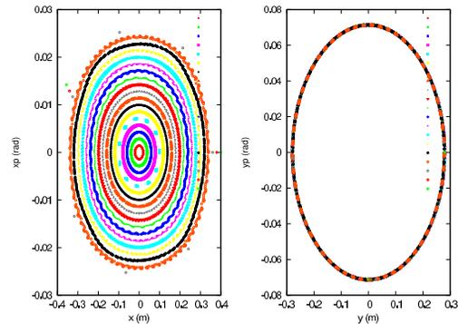
Figure 5: A scan in the  $(x, x')$  phase space is shown with a fixed initial value ( $y=28$  cm,  $y'=0$ ), for the linear optics ring. The left plot is a Poincaré map for the  $(x, x')$  section, showing a behaviour very close to elliptical curves even for large beam radii. The evolution of the other transverse coordinates  $(y, y')$  is totally decoupled, as can be inferred by the sharp ellipse in the right plot.
