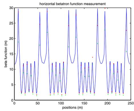
Figure 4: Red spots are the measured beta at BPMs after applying the overall scaling factors, while Green spots are not.
