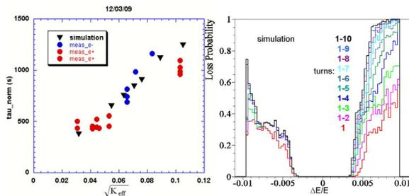
Figure 4: Left: calculated (black markers) and measured normalized lifetime for  $e^+$  (red dots) and  $e^-$  (blue dots) beams versus the square root of coupling. Right: simulated Touschek energy acceptance for ten turns.
