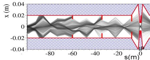
Figure 2: LER Touschek particles trajectories for the *Jan. '09 lattice* with three collimators rejecting particle losses.
