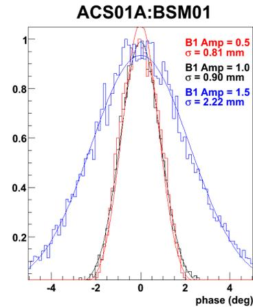
Figure 4: Longitudinal profiles at ACS01A calculated by IMPACT for Buncher 1 amplitudes of 50% (red), 100% (black) and 150% (blue) of the design amplitude.
