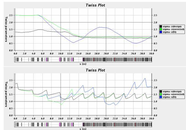
Figure 7: Design (black), fitted (green), and matched (blue) longitudinal (top) and horizontal (bottom) envelopes from MEBT2 to the entrance of ACS with Scheme C.
