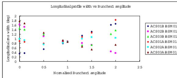
Figure 2: Longitudinal profile width in degrees of 324 MHz as a function of Buncher 1 amplitude.
