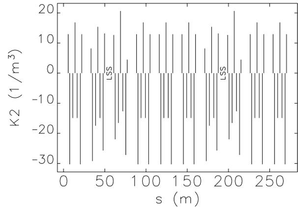
Figure 2: Sextupole distribution for a portion of the optimized 8LSS lattice.
