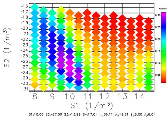
Figure 1: Output from sextupole scan used to optimize APS dynamic and momentum apertures.
