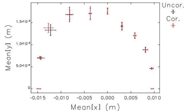
Figure 3: Dynamic aperture of optimized 8LSS lattice for 50 ensembles, with and without coupling correction.
