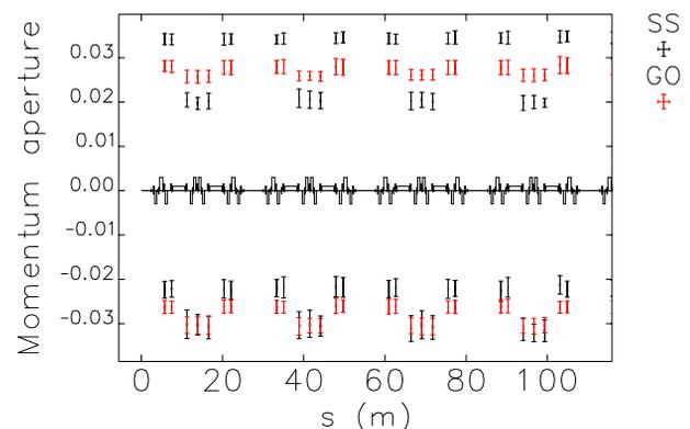
Figure 4: Comparison of momentum aperture for a portion of the lattice from the sextupole scan (SS) and genetic optimization (GO) methods. See text for explanation.
