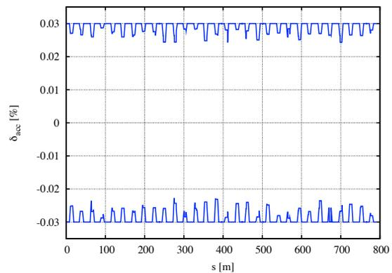
Figure 6: Momentum aperture with damping wigglers, three in-vacuum undulators,  $\pm 2.5$  mm vertical gaps, misalignment errors and field errors.
