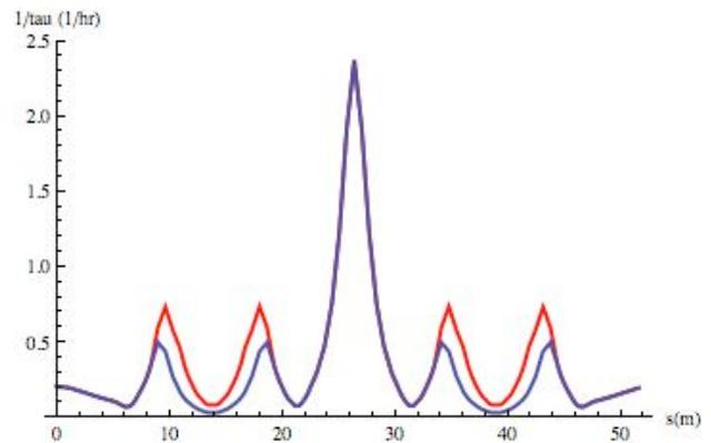
Figure 4: Local Touschek scattering rate for a single superperiod of the lattice. The straight sections have  $\delta_{acc} = 2.5\%$ . The dispersion region has  $\delta_{acc} = 2.5\%$  (blue),  $\delta_{acc} = 1.5\%$  (red). The total Touschek lifetimes are accordingly 3.3 and 2.9 hours.
