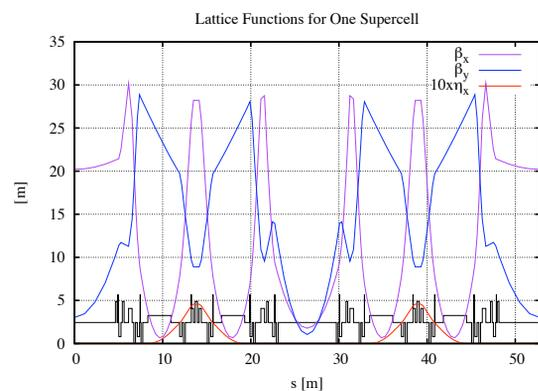
Figure 1: Twiss functions for one superperiod of lattice.
