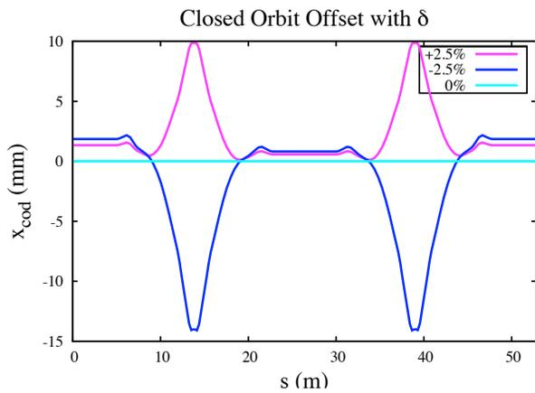
Figure 2: Dependence of horizontal closed orbit on momentum. One superperiod is shown.
