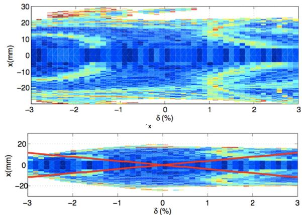
Figure 5: Off-momentum frequency map for lattice with no field errors and with systematic field errors in quadrupoles and sextupoles. The red lines show the scattering amplitude for particles in the dispersive region. The color represents the tune change on a log scale, with blue representing small change and orange substantial diffusion.
