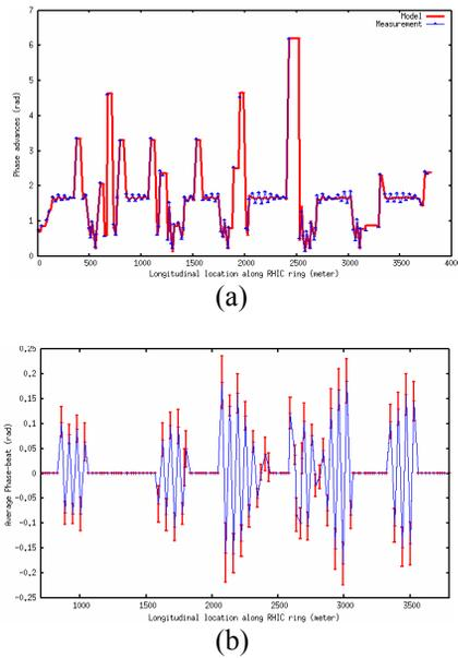
Figure 2: Phase beat measurement from the RHIC 2008 run. The abscissa is the location of the bpm's in units of meters and the ordinate is the phase in units of radians. (a) shows the result of one measurement. The red line is calculated from model and the blue dots are measured data. (b) shows the averaged phase beat of 5 measurements.
