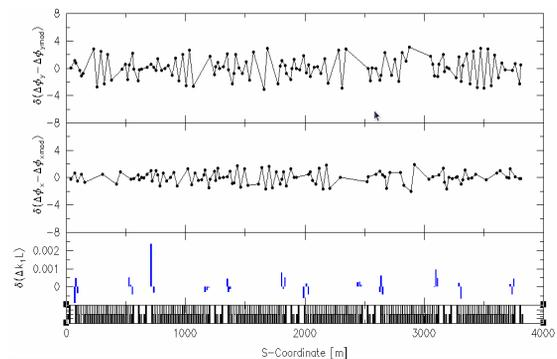
Figure 3: Experiment result in RHIC 2007 run. The top two graphs show the measured phase beat due to the preset trim quadrupole error and the bottom graph show the strengths of trim quadrupoles required to correct the phase beat as calculated from the SVD algorithm.
