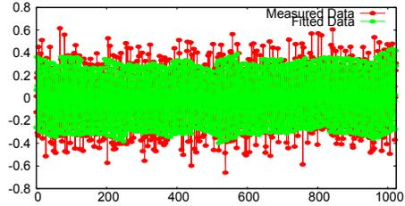
Figure 1: Example of excluded bpm data due to suspiciously large  $\chi^2$ . The red dots are measured data and the green line is the fitting result.
