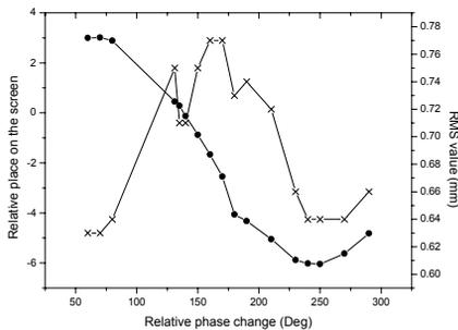
Figure 6: Centroid positions and beam sizes for different RF phase.
