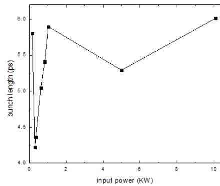
Figure 8: Bunch lengths for different input power.
