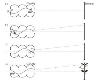
Figure 4: Bunch length measurement principle.
