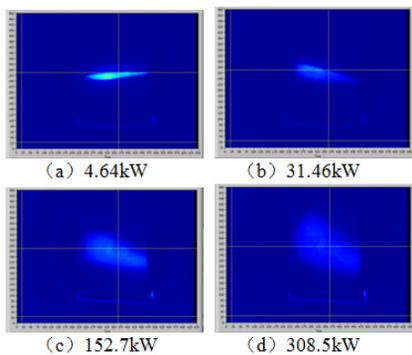
Figure 7: Beam spots for different input power.
