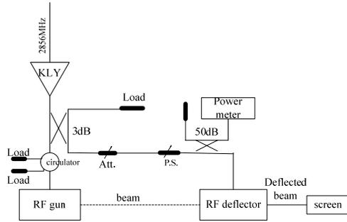
Figure 2: The power feed system sketch.
