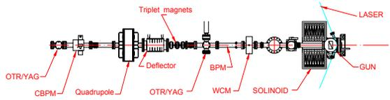
Figure 3: Layout of the bunch length measurement setup.
