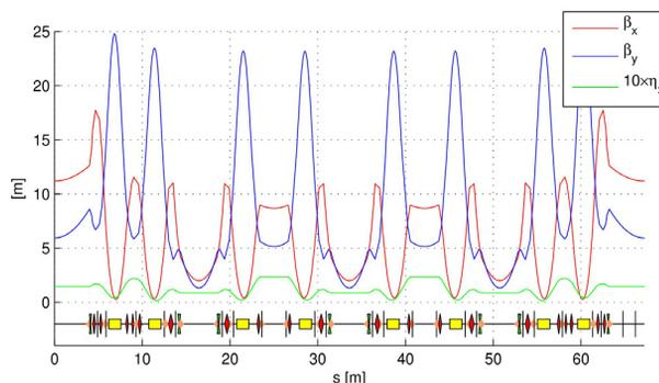
Figure 1: Optical functions for one quarter of the machine.
