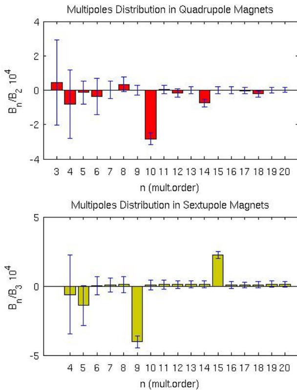
Figure 2: Normal high order multipole component for the quadrupoles (upper plot) and the sextupoles (lower plot). The solid bar corresponds to the average value all the measured magnets of a given type and the error bar to the standard deviation.
