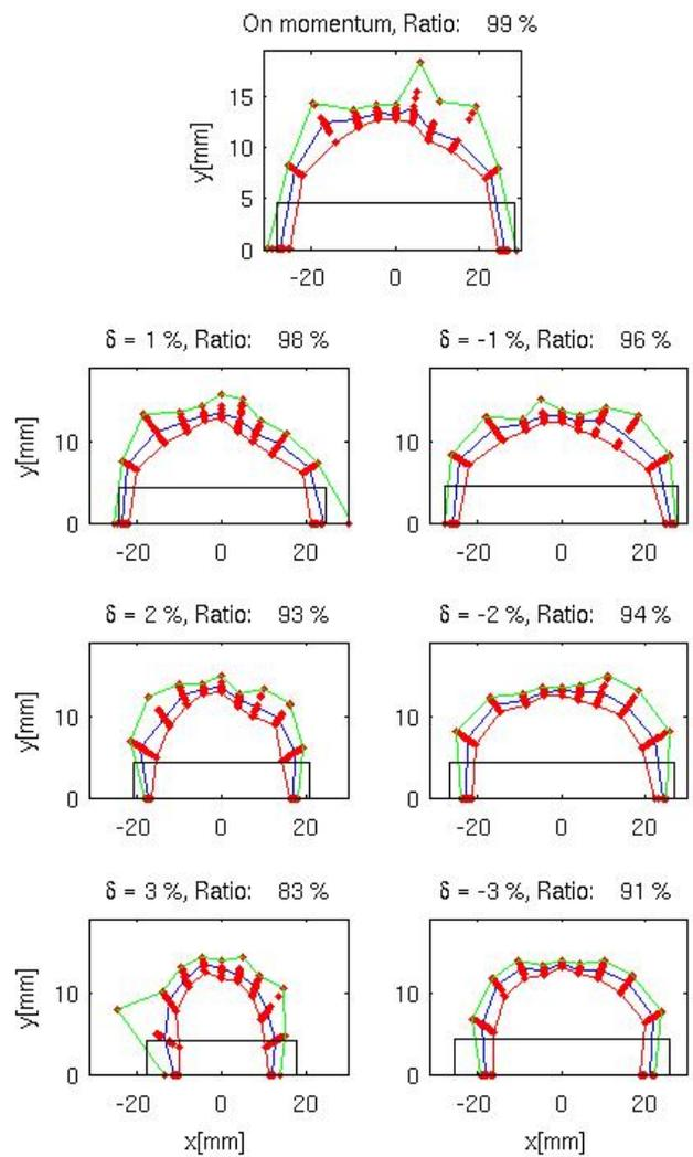
Figure 3: Dynamic aperture for 20 different sample machines at the injection point (s=0 in figure 1). The top figure is for the on energy particle, and each row for increasing values of the energy deviation. The green value is for the case with larger DA, the red for the one with smaller DA and the blue is for the average value. The black line is the projection of the physical aperture (excluding the septum). The percentage is the reduction of the DA respect the ideal case.
