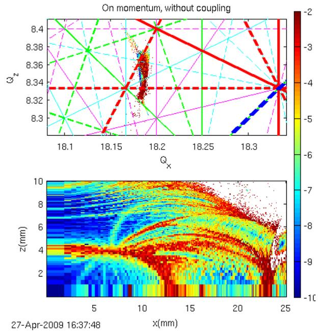
Figure 5: On energy frequency map for a sample case. The resonance visible at 12 mm is a third order  $2Q_x - Q_y = 28$
