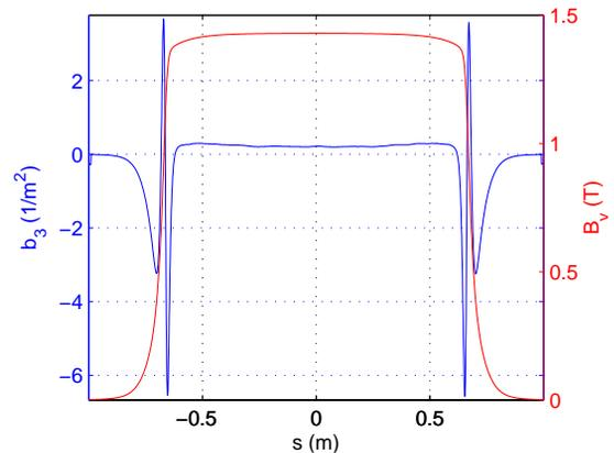
Figure 6: Sextupolar component (in blue) and dipolar component (in red) of the field in the bending magnet along the ideal trajectory of the electrons, for the reference bending magnet.
