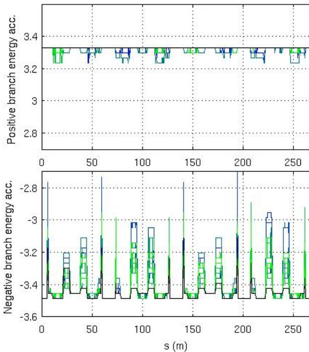
Figure 4: Local energy acceptance along the lattice. In order to provide the desired Touschek lifetime, it is required a 3% acceptance.
