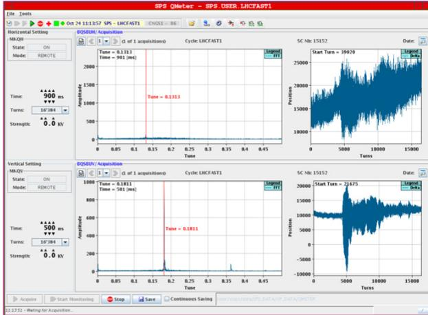
Figure 3: One of the applications used to kick the beam transversally and measure the tunes, called Qmeter: (upper left) horizontal tune and (lower left) vertical tune; (upper right) horizontal position and (lower right) vertical positions of the beam. Note the different timings.
