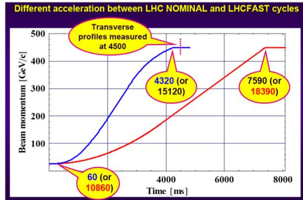
Figure 1: Comparison between the LHCFast cycle, which was used for the blow-up studies, and the nominal LHC cycle which will be used for LHC filling with nominal intensity bunch trains.
