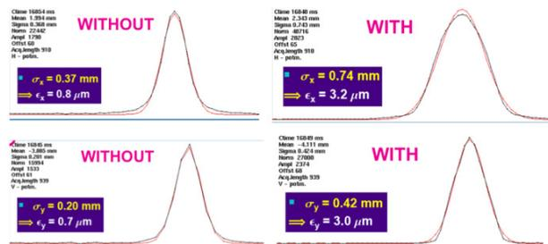
Figure 4: Transverse beam profile measurements using the wire scanners BWSH51995 and BWSV51995 at 4500 ms (see Fig. 1): horizontal/vertical profiles without and with controlled blow-up (upper/lower).
