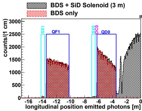
Figure 3: Longitudinal position of the emitted photons, red line are the photon emitted due to synchrotron radiation in the FFS only, black line shows the emitted photon when SiD field is superimposed.
