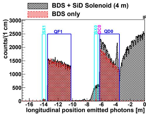
Figure 4: Longitudinal position of the emitted photons as in Fig. 3. The SiD magnetic field is scaled to fit a length of 4 m instead of 3 m.
