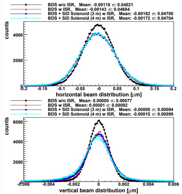
Figure 5: Beam distribution at the IP. For each of the case described in the text the mean and  $\sigma$  coming from the fit (drawn on the plot) are shown too.
