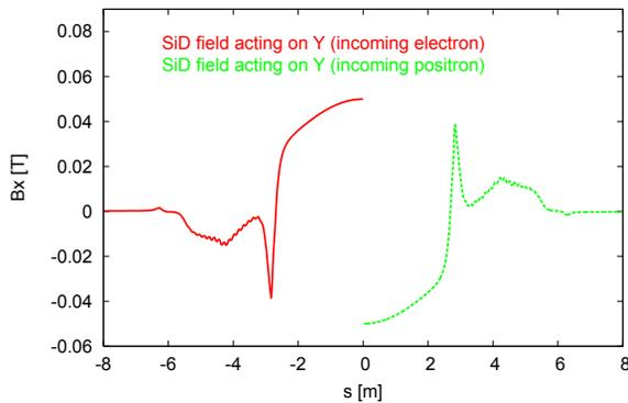
Figure 1: SiD fields acting on the vertical plane for an incoming electron (red-full line) and for an incoming positron (green-dashed line). IP is at  $s = 0$  m.  $B_x$  and  $s$  are in the beamline reference system.
