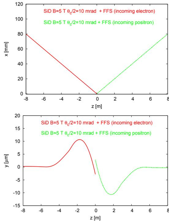
Figure 2: Electron (red-full line) and positron (green-dashed line) reference trajectories due to the last final focus magnets and the solenoid magnetic field. The horizontal plane (top) and vertical plane (bottom) are shown in the solenoid reference system.
