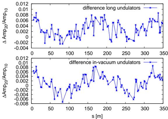
Figure 9: Plot showing the effect of the undulators on the  $\text{Amp}_{20}$ . Long undulator (top) and in-vacuum undulators (bottom).
