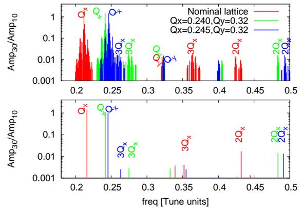
Figure 6: Frequency spectrum for horizontal tune approaching  $4^{\text{th}}$  order resonance. For measured (top) and simulation taking into account the decoherence (bottom).
