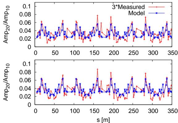
Figure 5: Normalized  $\text{Amp}_{20}$  for  $Q_x = 0.21$  (top) and  $Q_x = 0.273$  (bottom).
