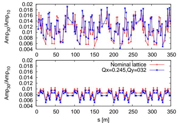
Figure 7: Normalized  $\text{Amp}_{30}$  for measured (top) and simulation (bottom) approaching  $4^{\text{th}}$  order resonance.
