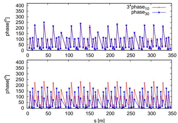
Figure 8:  $\text{Phase}_{10}$  and  $\text{Phase}_{30}$  plotted versus longitudinal location for both measured (top) and simulation (bottom) for  $Q_x = 0.21$ .
