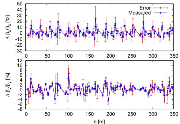
Figure 3: Beta-beat for horizontal (top) and vertical direction (bottom). Maximum beta-beat of  $\sim 6\%$  and  $\sim 20\%$ , respectively in vertical and horizontal planes.
