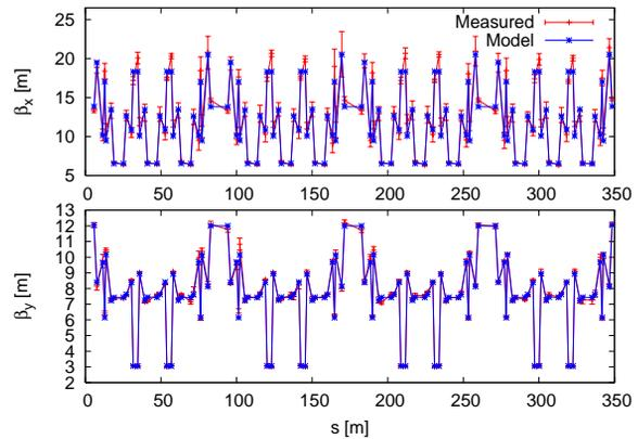
Figure 2: Measured and model betatron function for horizontal (top) and vertical (bottom) planes. The superperiodicity of the ring is four.
