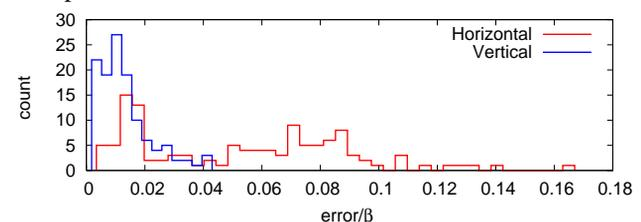
Figure 4: Histogram of the beta function error bar normalized to the beta.
