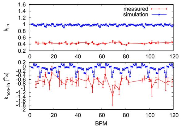
Figure 10: Linear and non-linear factor for BPM non-linearity in the horizontal plane.
