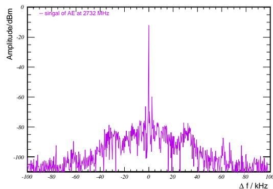
Figure 4: Spectrum of the AE at the 2732 MHz revolution harmonic showing the upper and lower first synchrotron sideband. The second sideband is just visible. The spectrum was recorded with a resolution bandwidth of 100 Hz and for a span of 200 kHz.
