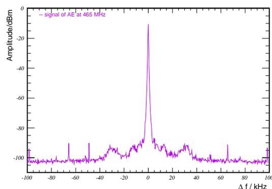
Figure 5: Spectrum of the AE at the 465 MHz revolution harmonic showing the upper and lower first synchrotron sideband. The second sideband is not visible. The spectrum was recorded with a resolution bandwidth of 300 Hz and for a span of 200 kHz with video averaging turned on.
