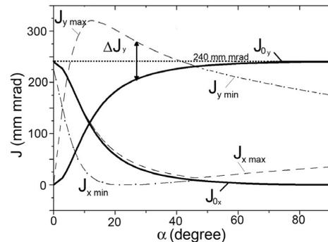
Figure 2: Action variables without harmonic sextupole correction.  $\Delta p/p=0$ .
