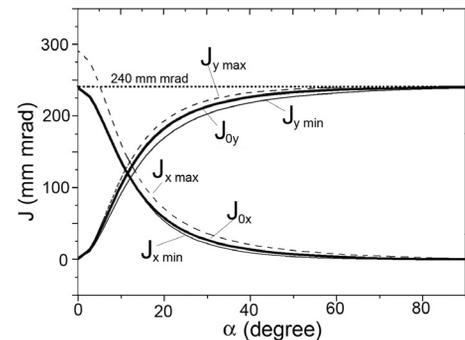
Figure 3: Action variables after correction with harmonic sextupole.  $\Delta p/p=0$ .
