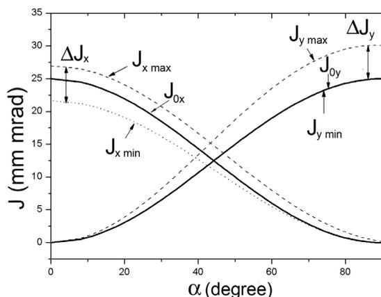
Figure 5: Action variables in the RESR for the accumulation orbit with  $\Delta p/p = +0.8\%$ .
