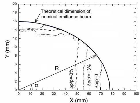
Figure 4: Limit of beam survival with real aperture limits.
