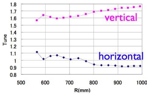
Figure 2: Tune variation with accelerator radius
