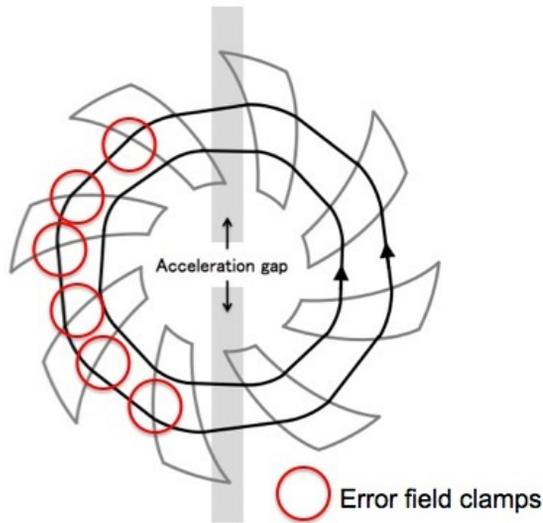
Figure 3: Distribution of error-field clamp: The gap of field-clamps checked with open circles were 10 mm wider than the others.
