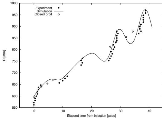
Figure 6: Result of beam measurement with an acceleration speed of 3.5 kV/turn. Closed circles and open circles stand for the experimental result and closed orbit derived from beam tracking simulation, respectively. Results of tracking simulation is presented with the solid line.
