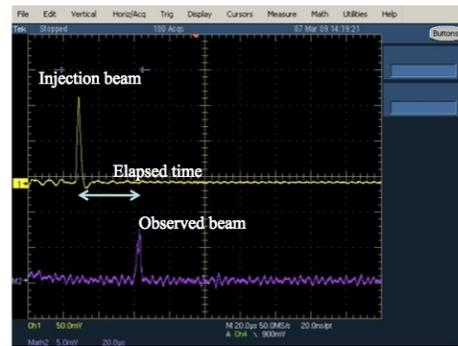
Figure 5: Beam measurement using a radial probe: Top signal is the beam at ion source. Bottom signal is the beam observed with the radial probe.
