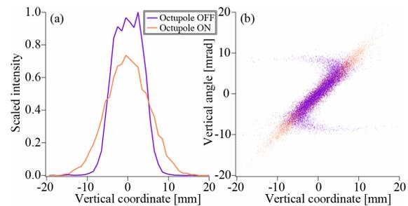
Figure 5: Real-space and phase-space distributions of the beam on the target obtained by single-particle tracking based on the beam optics in Fig. 4. The ion species is 6.4 MeV/u  $^{14}\text{N}^{6+}$  with the rms emittance of  $6\pi$  mm mrad.
