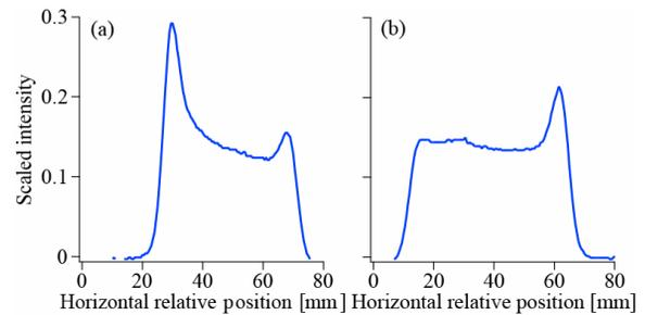
Figure 3: 1D intensity distributions measured on the target, indicating the effect of the beam centroid displacement (a) and sextupole field (b).
