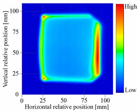
Figure 2: 2D intensity distribution of a 10 MeV proton beam on the target. The relative intensity of the beam is obtained from the optical density of the irradiated GAFCHROMIC film.
