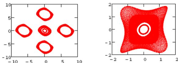
Figure 4: X (left) and Y(right) phase spaces for 25 percent beta-function difference.
