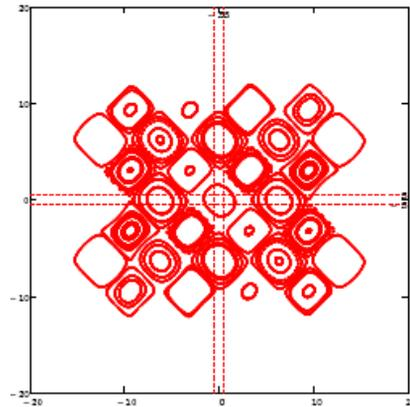
Figure 2: Phase space of the 1-cell map with periodic integrable lens.
