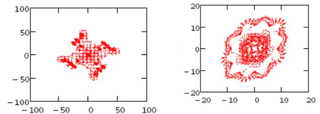
Figure 5: X (left) and Y(right) phase spaces showing a chaotic net in between of islands with regular motion. One can see that the particle wanders between the regions with stable motion and its amplitude grows in a diffusion-like manner to very large values.
