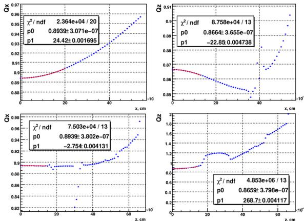
Figure 1: Tune-amplitude dependence for the sextupoles.
