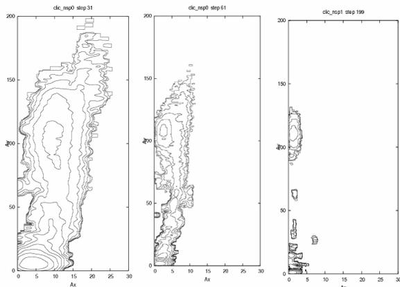
Figure 4: Particle distribution for 3100, 6100 and 19900 turns; scale is  $30 \times 200$  rms beam size at extraction.
