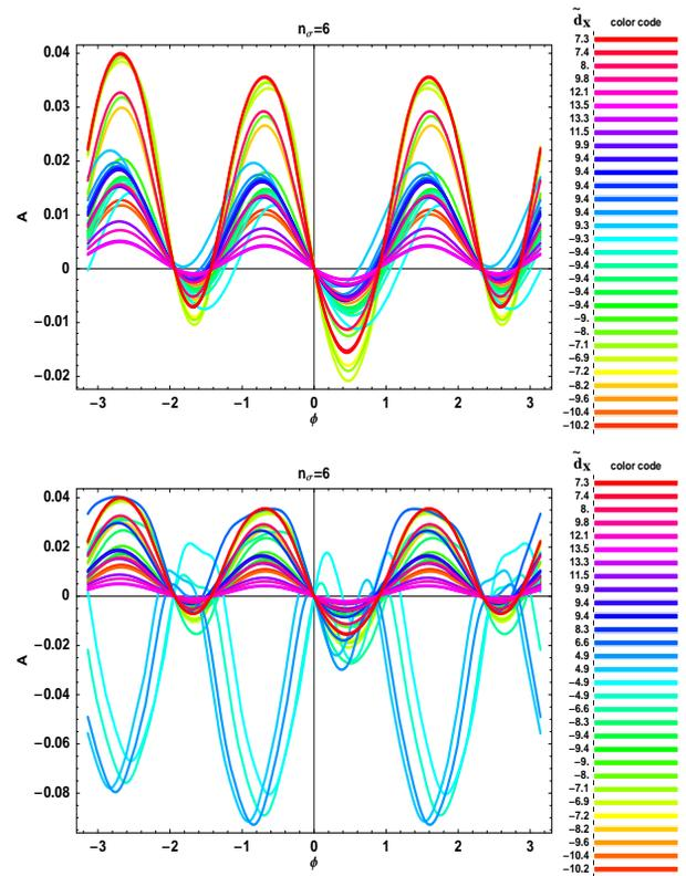
Figure 6: Individual contributions to  $\tilde{h}$  of the 30 long-range collisions near IP5 (horizontal crossing) for two scenarios: nominal (top) and early separation [7] (bottom).
