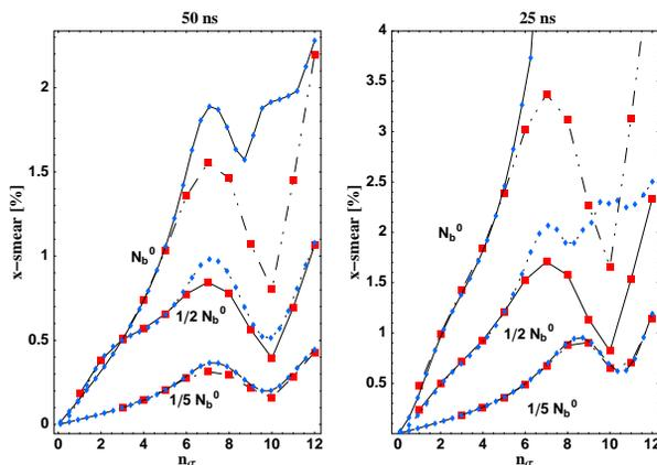
Figure 5: Agreement between Lie-algebra model (red) and Sixtrack (blue) for increasing bunch population  $N_b$  and two LHC collision schemes “50 ns” and “25 ns” (head-on is included). The curves correspond to 1,  $1/2$  and  $1/5$  times the nominal bunch population  $N_b^0 = 1.15 \cdot 10^{11}$ .
