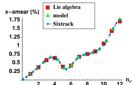
Figure 4: Agreement between Lie algebra, tracking model and Sixtrack for a sample set of long-range collisions in the LHC. Shown is smear of the horizontal emittance computed over  $2^{10}$  turns as a function of initial  $x = n_\sigma\sigma$ .
