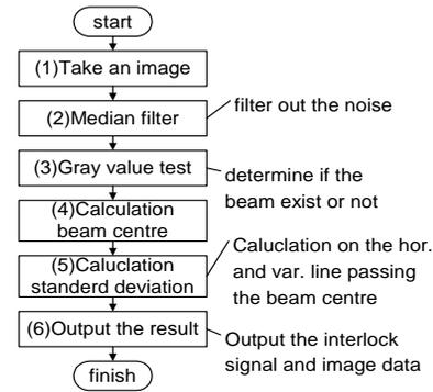
Figure 2: The flow chart of image processing.
