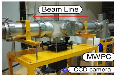
Figure 1: Screen monitor system and MWPC monitor.
