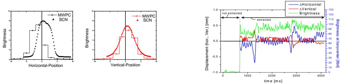
Figure 4: Both horizontal and vertical beam profile measured by the SCN and MWPC.
