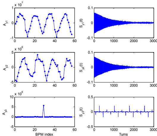
Figure 8: ICA decomposition for vertical S1-S3 modes.
