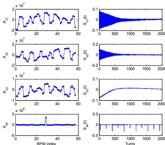
Figure 9: ICA decomposition for horizontal S1-S4 modes.
