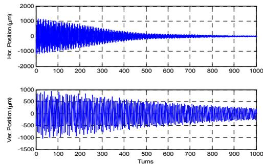
Figure 1: Betatron oscillation excited by kicker. Synchrotron oscillation excited by positive longitudinal feedback. It is R6BPM7 turn-by-turn data.
