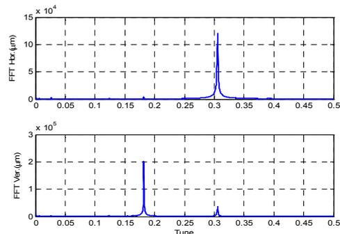
Figure 2: Spectrum of the above turn-by-turn data. Horizontal betatron tune is around 0.295 Vertical is 0.1817. Synchrotron tune is 0.0133
