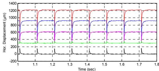
Figure 5: Orbit motions of 5 BPM during injection caused by kicker and septum.
