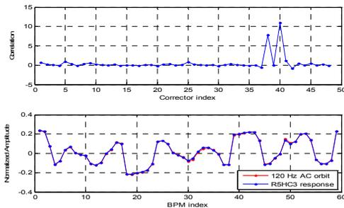
Figure 10: The above figure is correlation between 120 horizontal AC orbit versus all horizontal correctors. The below one shows the AC orbit and its most relevant corrector (R5HC3) response.
