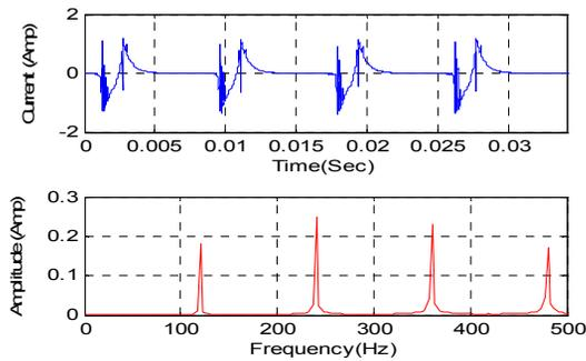
Figure 3: Superconducting wiggler power supply current readings and its spectra amplitude.
