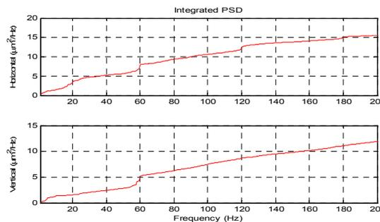
Figure 1: Integrated orbit stability before horizontal power supply upgrade.
