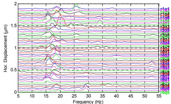
Figure 7: Quadrupole horizontal vibration.
