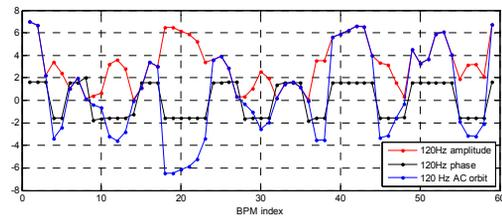
Figure 9: 120 Hz horizontal BPM amplitude, phase and AC orbit.
