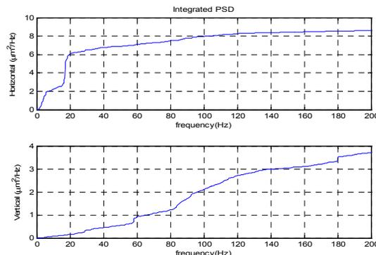
Figure 2: Integrated orbit stability after horizontal power supply upgrade.
