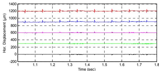
Figure 6: Orbit motions of 5 BPM during injection caused by kicker only.
