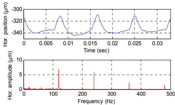
Figure 4: Orbit motion due to the ill superconducting wiggler power supply.
