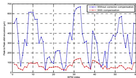
Figure 11: Maximum orbit excursion amplitude due to septum and compensated by the correctors.
