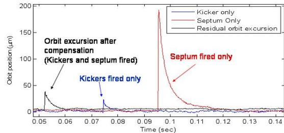
Figure 12: Orbit excursion of R6B7 due to septum only, kickers only and the residual orbit after compensation by the dedicated corrector.
