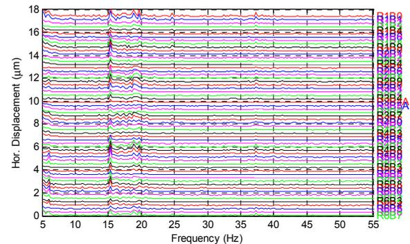
Figure 8: Horizontal orbit motion spectrum. The noise spreading between 15~25 Hz is correlated to the ground vibration.
